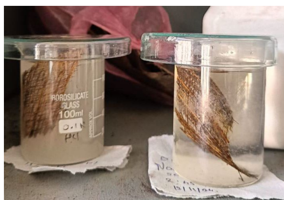
Figure 2. Chemical softening with NaOH and Na 2 CO 3
